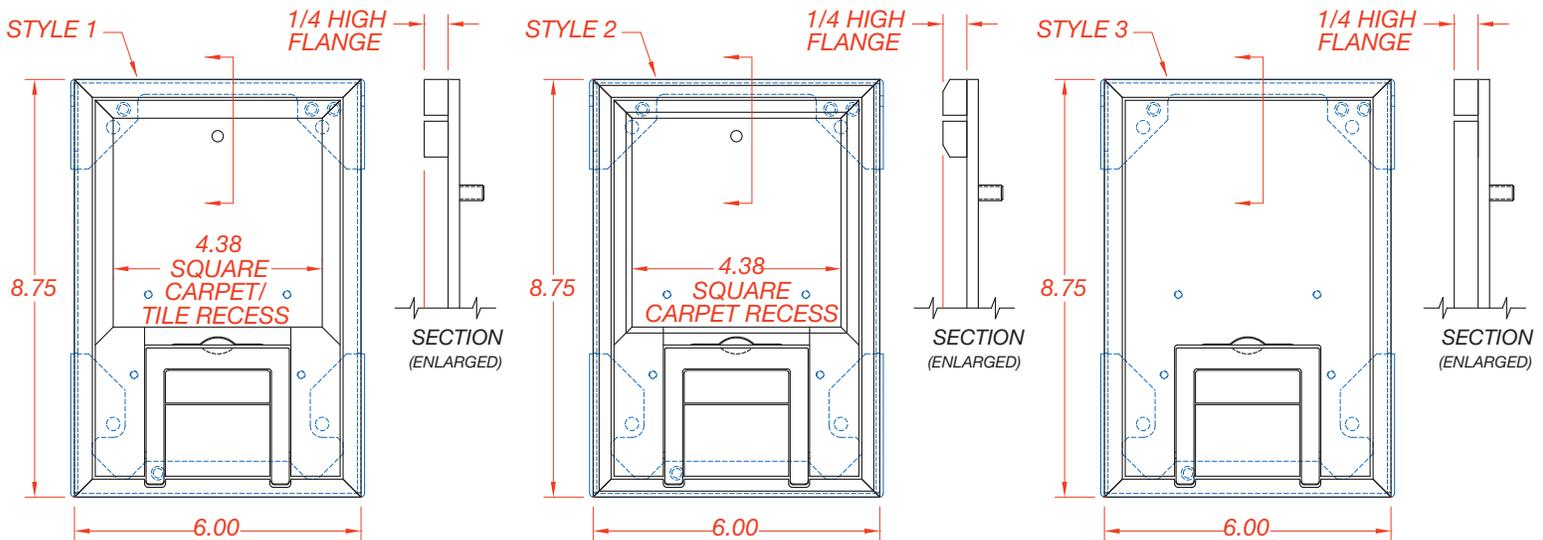
**\*\*Note:** Cover Shim Kit (FL-200-CSK) may be required to set the height of box "Pre-Pour" so the top of Finish Cover matches top of finished floor.
